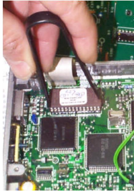
REMOVE THE CHIP USING A REMOVAL TOOL. TRY RADIO SHACK IF YOU DON'T HAVE ONE.
