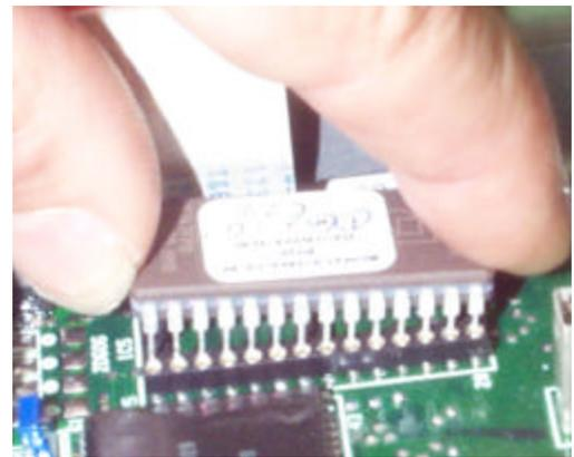
INSERT THE FRONT ROW OF PINS AND PUSH CHIP FULLY INTO THE SOCKET. INSPECT THAT ALL PINS ARE IN THEIR SOCKETS.
